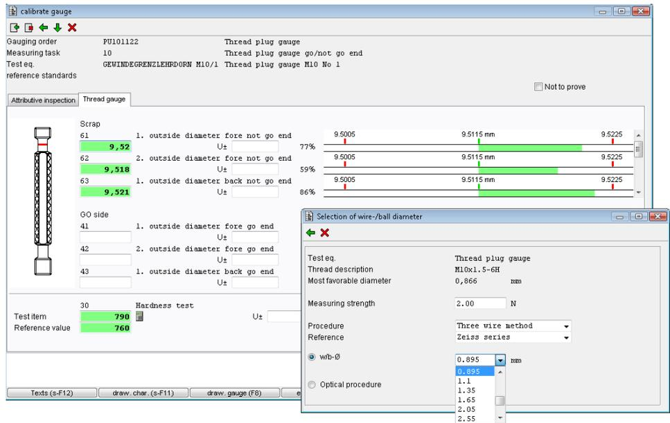
Furthermore there is a variety of more gauges for which no standardized inspection directives are available. The following chart shows all those gauges for which all arrangements have been made, also without any planning, in order to start calibration immediately. Tolerances can be indicated through an easy chart system.
